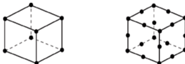
Figure 4.2 - Representation of a linear element 8-node brick, C3D8 (left) and a quadratic element 20-node brick, C3D20 (right).
