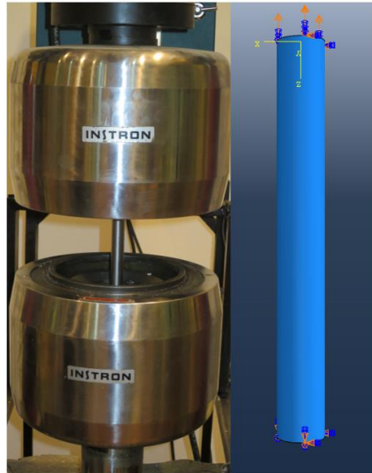
Figure 4.3 - Photo of 15PIN235 before the test (left); geometry and boundary conditions of the corresponding numerical model in Abaqus/CAE .
